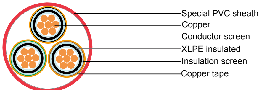
XLPE Insulated Cable to IEC 60502-2
