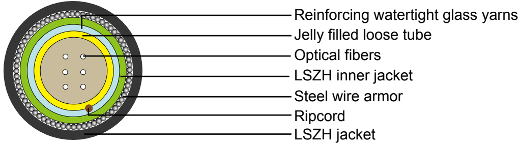
Steel Wire Armored Optical Fiber Cable with LSZH Sheath
