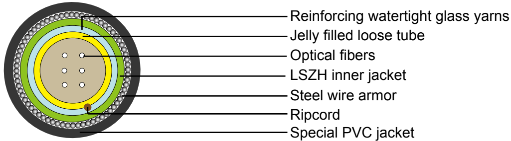
Steel Wire Armored Optical Fiber Cable
